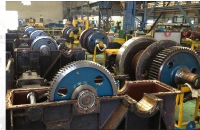
Mooring Winch Overhauling
