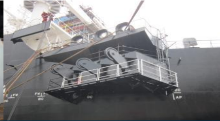
Roller Fairlead Fabrication and Installation
