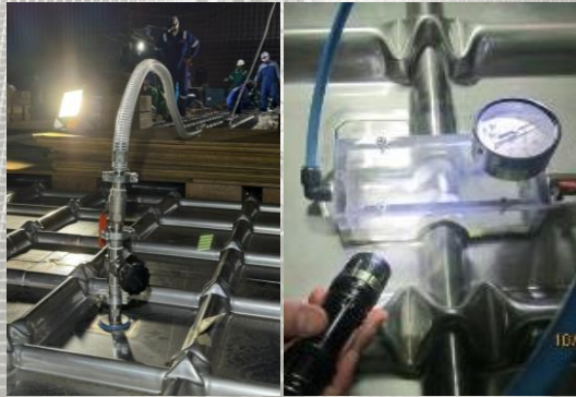
Vacuum and Local Helium Test
