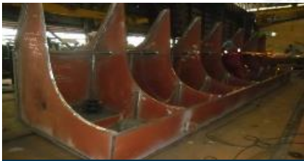
Fabrication Mooring Fairlead Foundation
