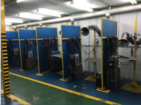
95 m 2 area with 10 welder stations
