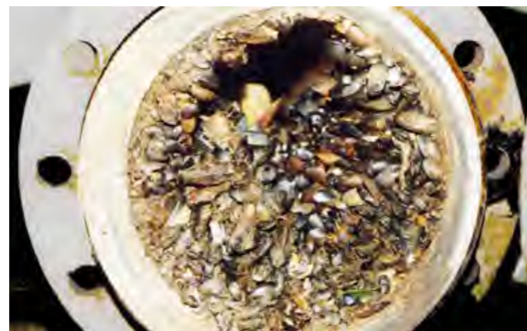
VESSEL PIPES WITHOUT MGPS PROTECTIO
