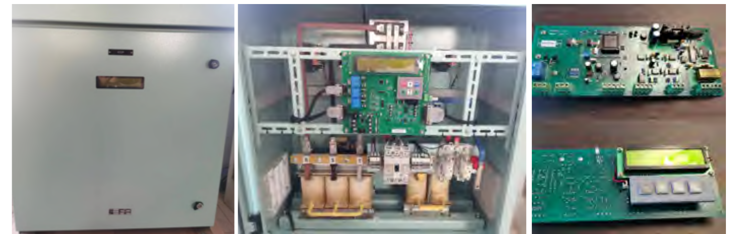
ICCP POWER CONTROL UNIT
